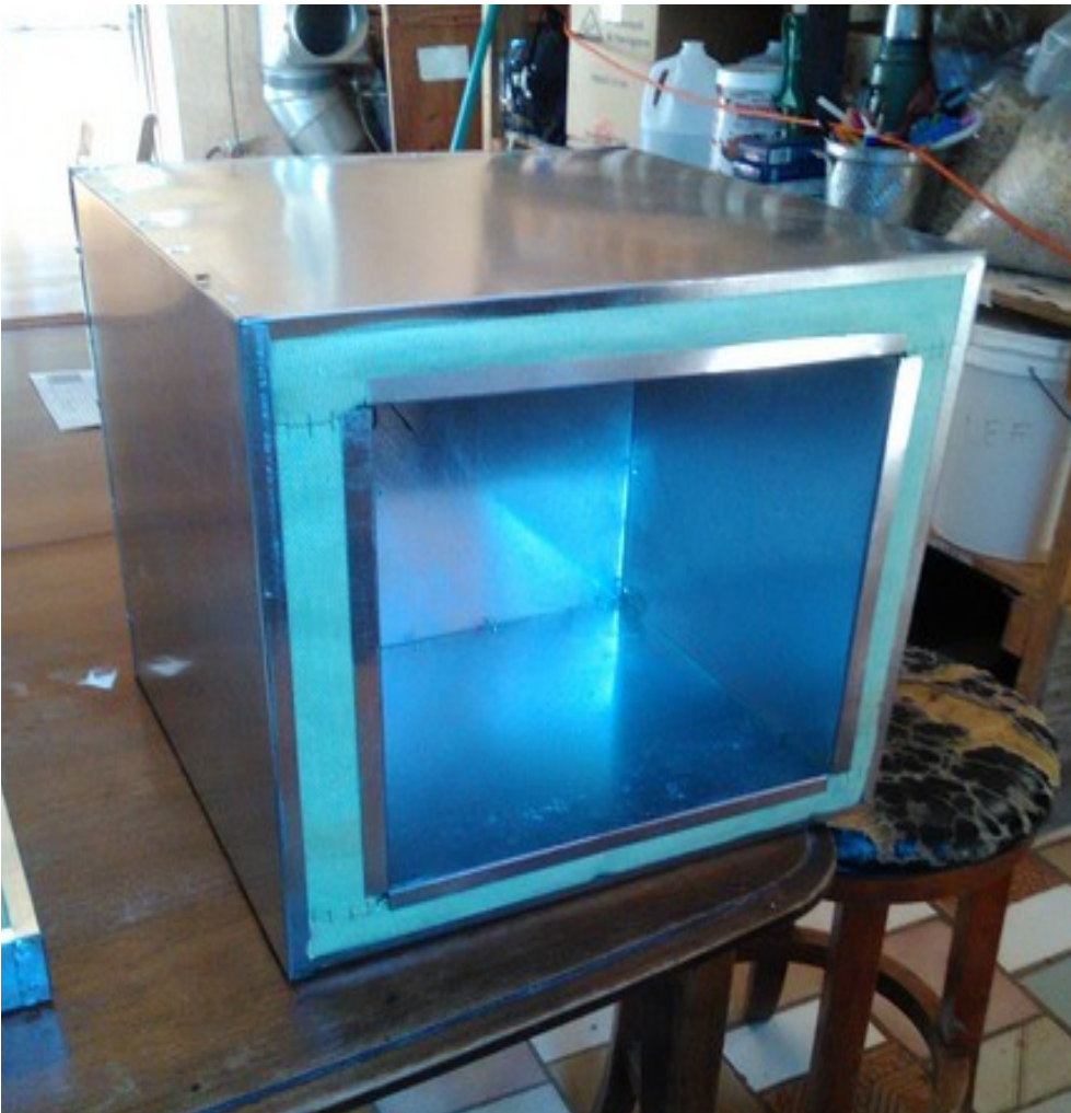
Roxy Metallica with a metal inner oven and an exterior metal covering.
