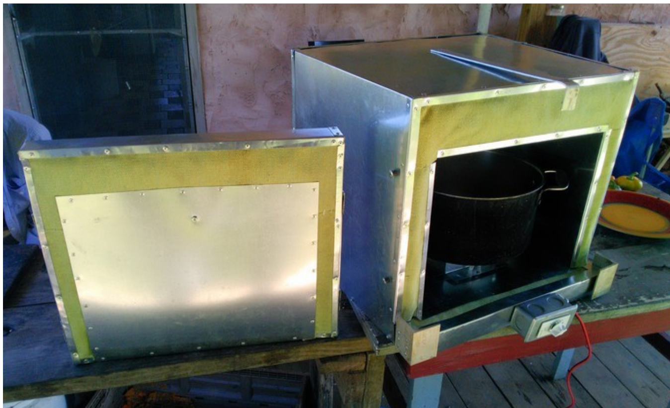
Roxy Deluxe looks and functions very much like a “real” oven. It can be set up to run at a wide range of power levels. It has a door that is easily set in place.
