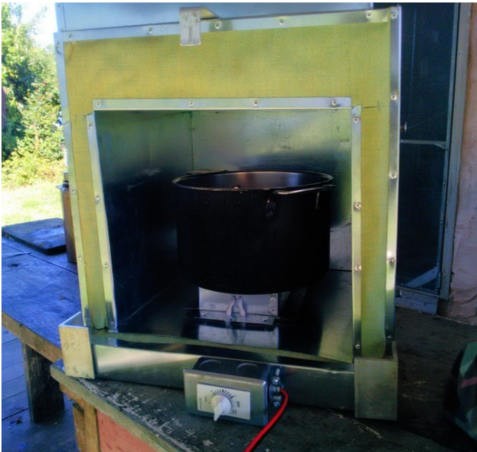
Roxy Deluxe is large enough for a large pot. The timer in front turns it off after the cooking is done. This is the fanciest solar cooker we have built.
